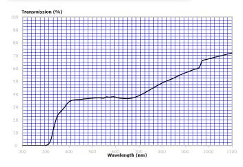
A Linear Polarizer has a typical transmission of 38% while blocking 62% of the light not in the polarization plane.
