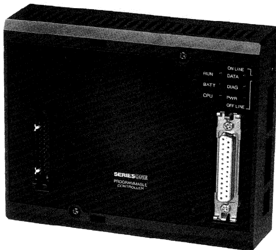
Figure 2.9 DATA COMMUNICATIONS UNIT
