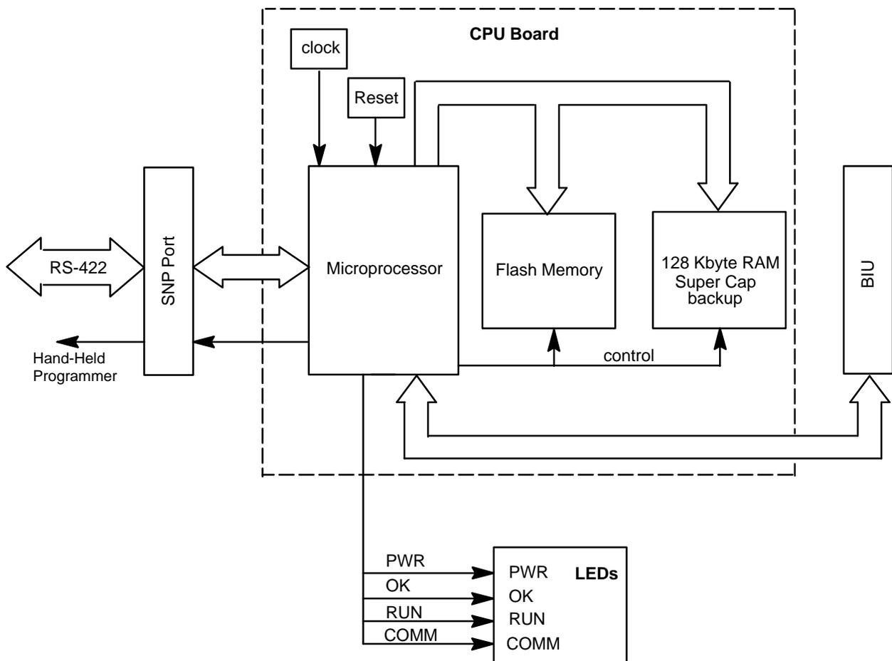
Figure 1-4. Micro Field Processor Functional Block Diagram
