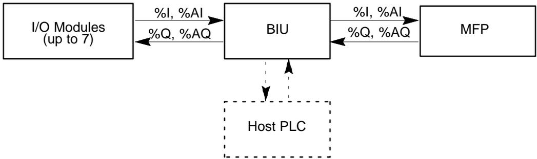
Figure 1-2. Field Control Station Block Diagram
