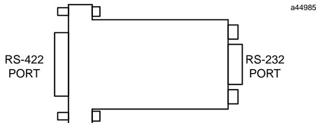
Figure 2-5. Series 90 SNP to RS-232 Adapter
