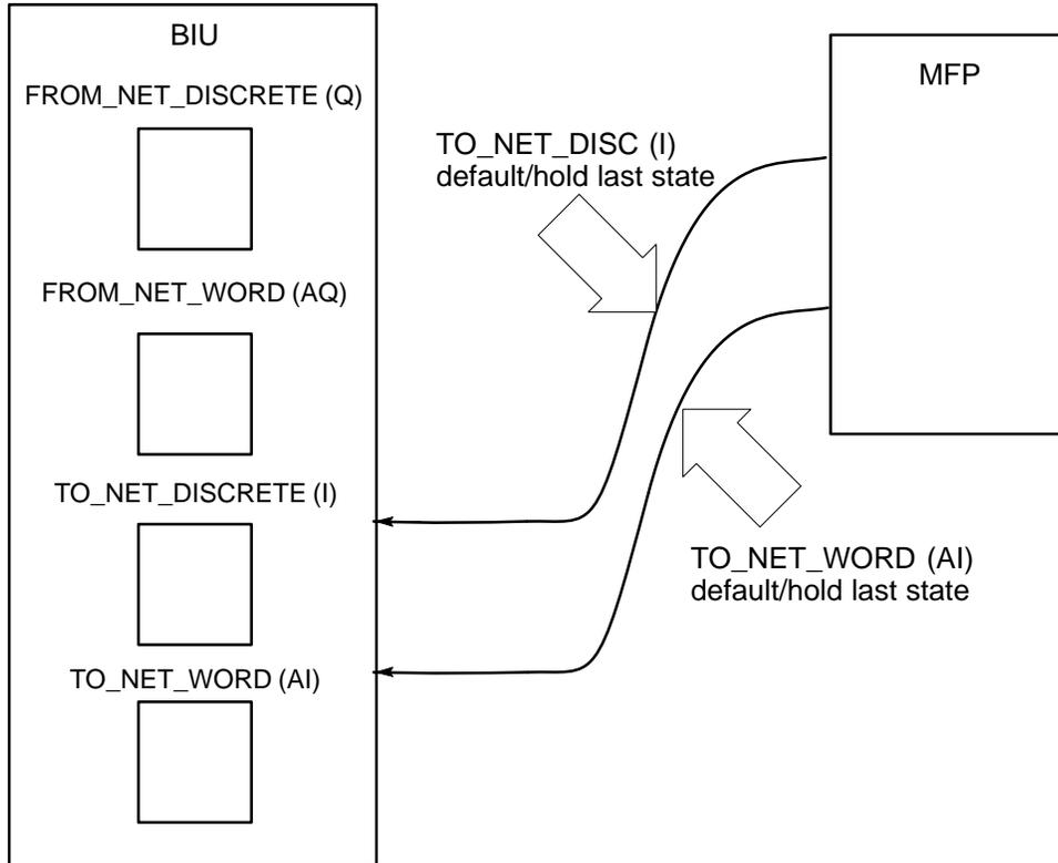
Figure 3-10. Default/Hold Last State Configuration Parameters for BIU Inputs
