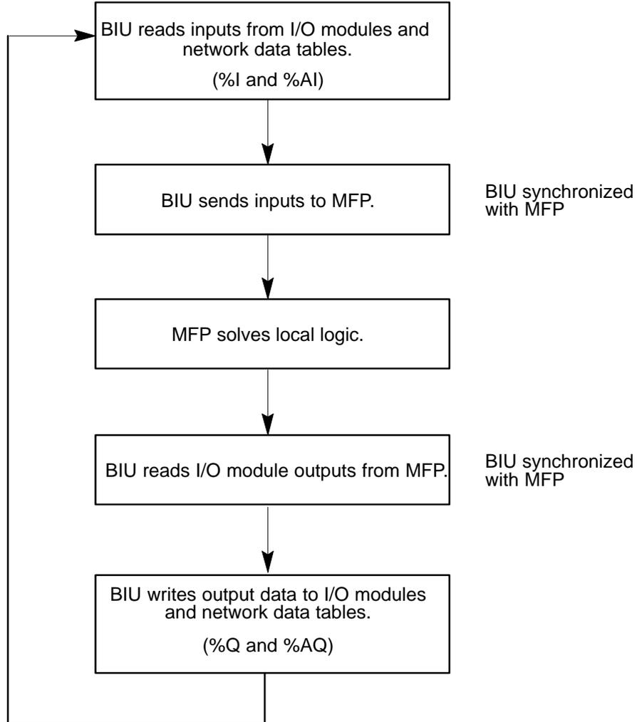
Figure 1-3. Overview of MFP Interaction with the BIU
