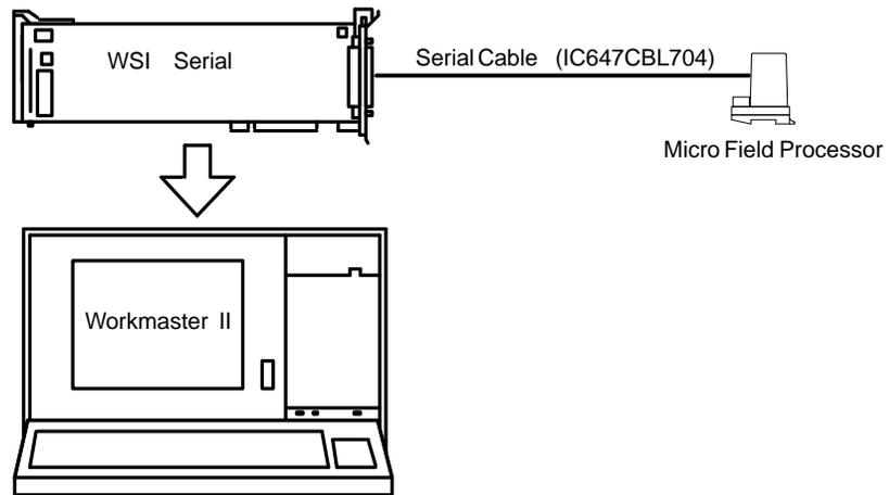
Figure 2-3. Logicmaster 90 Programmer to MFP Connection through a WSI
