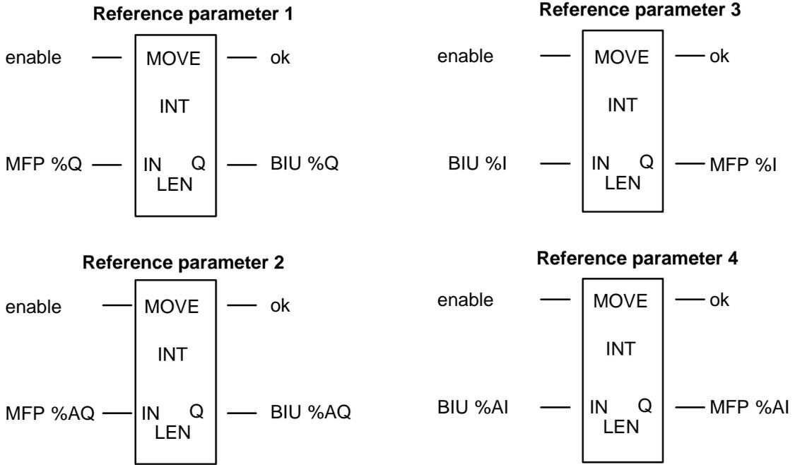
Figure 3-7. Move Function Blocks for Example 3
