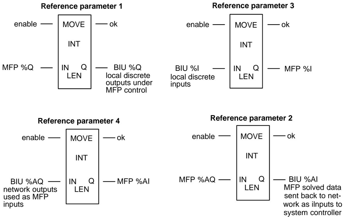
Figure 3-5. Move Function Blocks for Example 2
