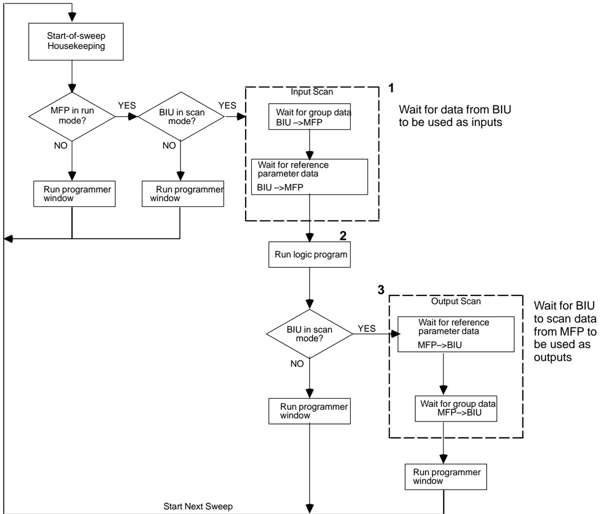
Figure 5-1. Micro Field Processor Synchronous Sweep
