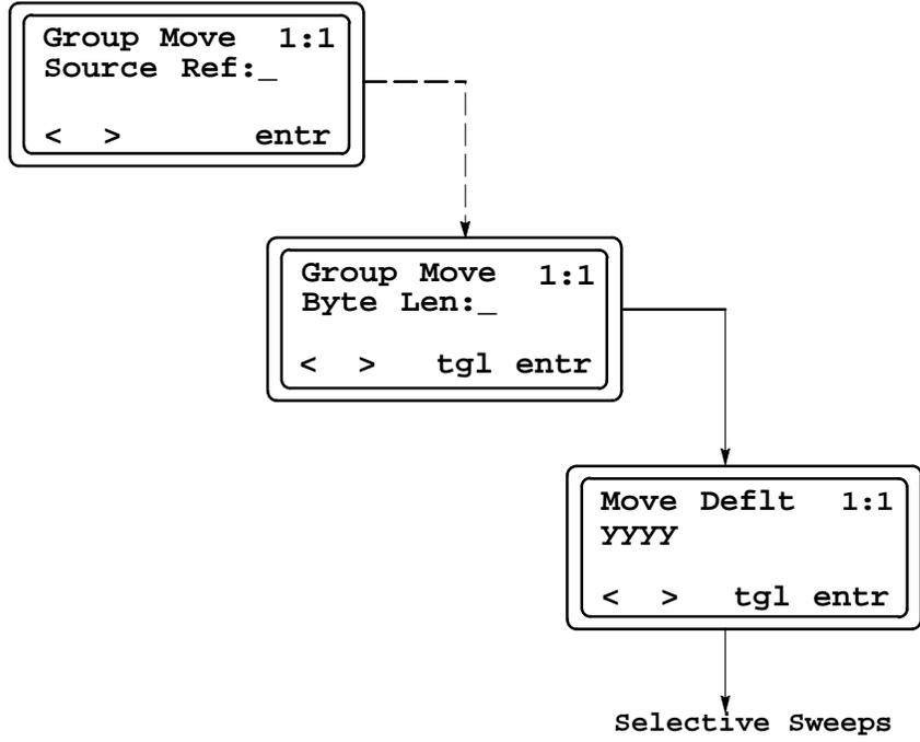
Figure 3-12. Group Data Move Configuration Process
