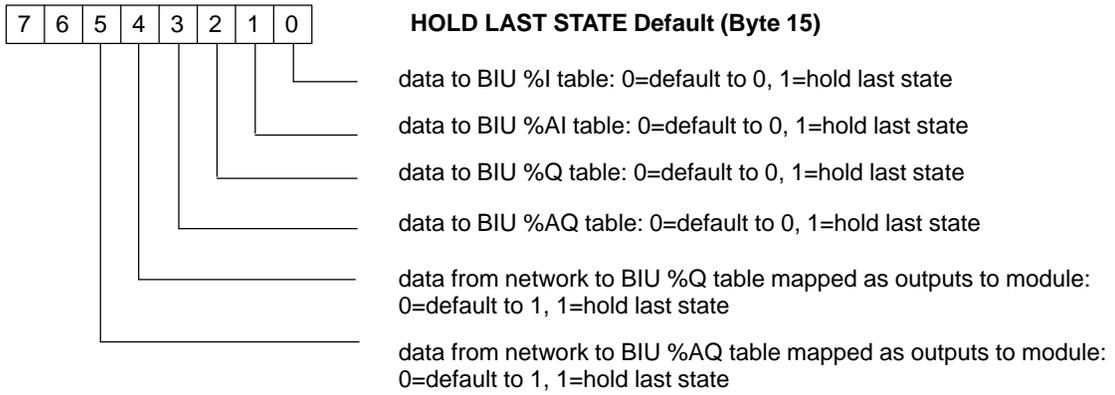
**Figure 4-1. Bit Map for Hold Last State Default Byte**
