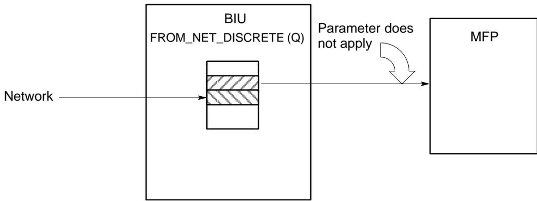
Figure 3-9. Case Where Default/Hold Last State Parameter Does Not Apply
