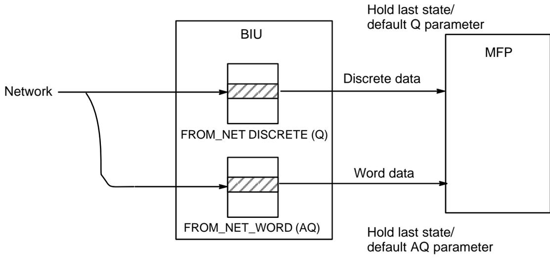
Figure 3-8. Default/Hold Last State Configuration Parameters for BIU Outputs
