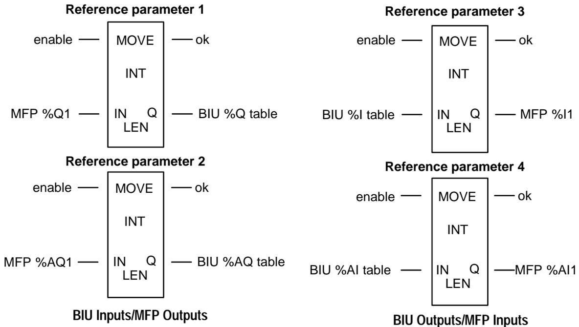
Figure 3-1. BIU Reference Parameters Described as Data Move Function Blocks
