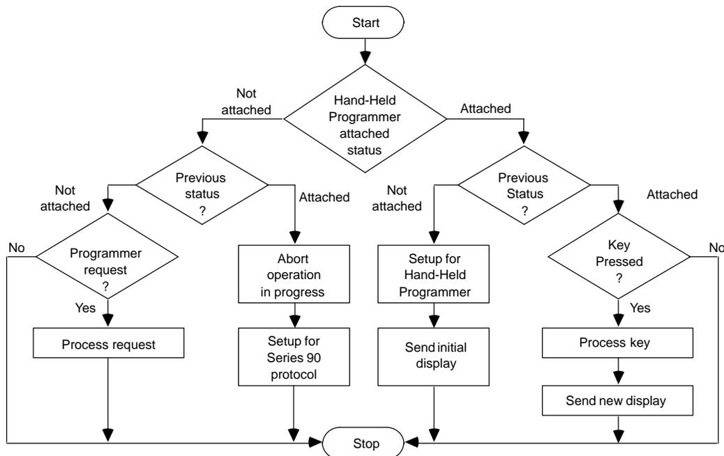
Figure 5-2. Programmer Communications Window Flow Chart
