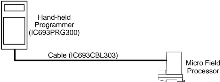
Figure 2-2. Hand-Held Programmer Cable Connection to a Micro Field Processor
