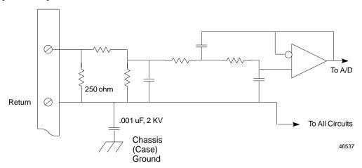
The module stores the most recent 16 samples for each channel in a buffer. The outputs of the buffer amplifiers are sequentially connected by an analog multiplexer to a 16-bit A/D converter. All channels are converted approximately once every millisecond.. The input span of the A/D is fixed, presenting binary values of 0 to 65535 for 0 to 25 milliAmps, with one LSB = 0.38 microAmps.
