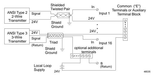
If the module is installed on an I/O Terminal Block with Box Terminals or Barrier Terminals, an Auxiliary Terminal Block can be used as shown to provide the additional wiring terminals. For the I/O Terminal Block with Wire to Board Connectors, external connection points are usually preferred, although an Auxiliary Terminal Block can be used. Auxiliary Terminal Blocks have all terminals connected together internally.
