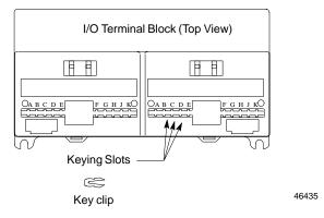
Refer to the following table for keying locations for various types of I/O modules. The check marks in the table correspond to the keying slots in the I/O Terminal Block.
