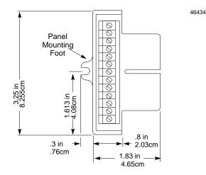
The I/O Terminal Block must be mounted on the DIN rail before installing an Auxiliary Terminal Block.
