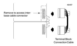
The <u>connectors are keyed</u> to assure proper installation. After installing the cable, be sure it is firmly seated on both connectors.
