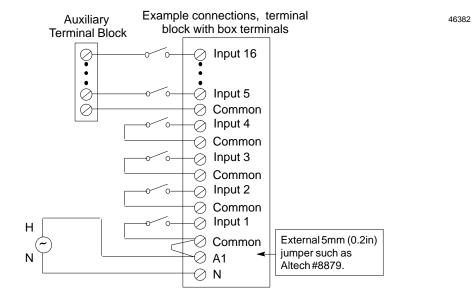
For an I/O Terminal Block with Barrier Terminals or an I/O Terminal Block with Wire to Board Connectors, an Auxiliary Terminal Block with Barrier Terminals might be connected as shown in the following example.
