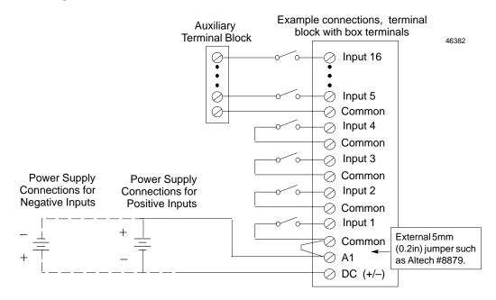
For an I/O Terminal Block with Barrier Terminals, an Auxiliary Terminal Block with Barrier Terminals might be connected as shown in the following example.
