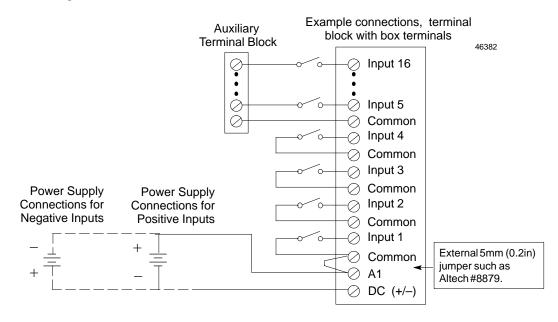
For an I/O Terminal Block with Barrier Terminals, an Auxiliary Terminal Block with Barrier Terminals might be connected as shown in the following example.
