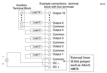
For an I/O Terminal Block with Barrier Terminals or an I/O Terminal Block with Wire to Board Connectors, an Auxiliary Terminal Block with Barrier Terminals might be connected as shown in the following example.
