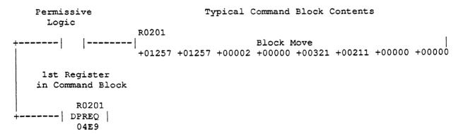
The exact content of the Command Block depends upon the type of command it describes, as summarized below. In this discussion, the term "Register 1" simply means the first register of a group. Register 2 is the second register, and so on.
