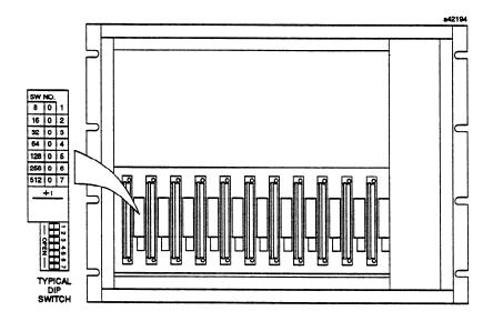
The Reference Number assigned to each Bus Controller is a beginning address in the I/O Table where the Bus Controller's input and output data will be located. This data includes diagnostics and command information.
