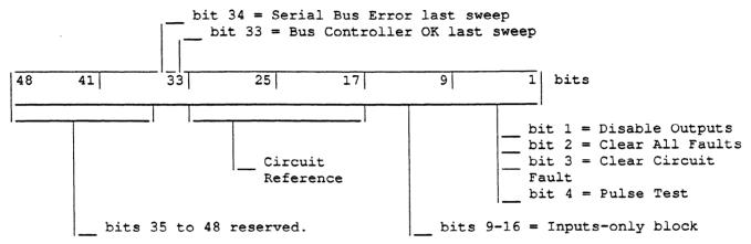
Bits 1 - 4 are used for commands. Bits 9 - 32 are used only for the Clear Circuit Fault command; they contain the circuit reference of the fault, and its I/O type.
