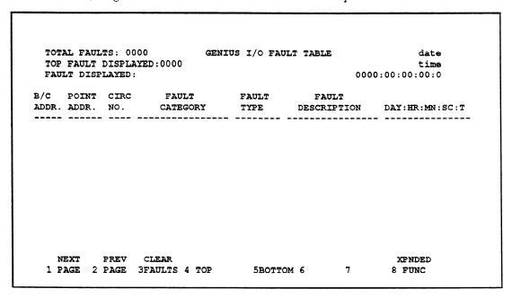
This screen can only be displayed if the current ladder logic program includes the CPU Configuration function, and if Genius I/O diagnostics is enabled in the CPU Configuration Set Up Menu.
