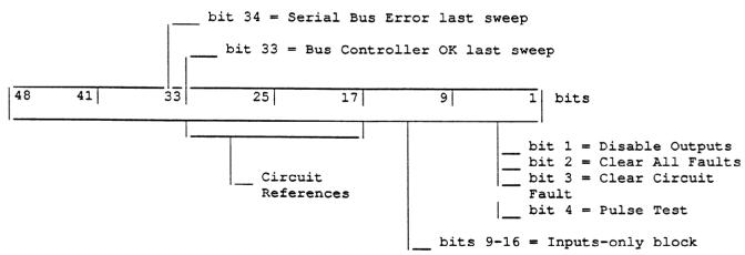
Before clearing Bus Controller input bit 1, the CPU copies it into Bus Controller output bit 33. On the next sweep, if the Bus Controller fails to reset input reference bit 1 to 1, the CPU looks at output reference bit 33. If bit 33 was 1 on the previous sweep, a Bus Controller fault is triggered. If it was 0 on the previous sweep, no additional fault occurs.
