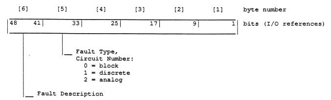
Fault 1 is an I/O circuit fault. Its fault type and description would be stored in R141. Moving the cursor to R141 would show the binary content of this register:
