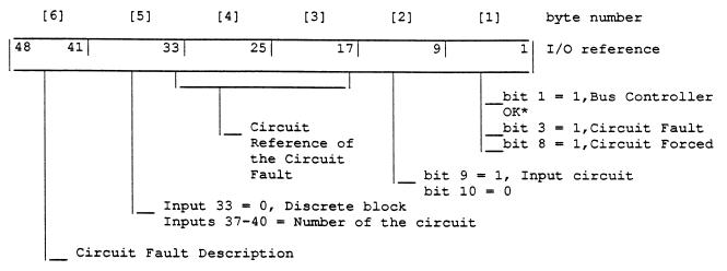
\* Automatically cleared by the CPU if DIAGNOSTICS ENABLED is set to Y on the CPU Configuration Setup Menu.
