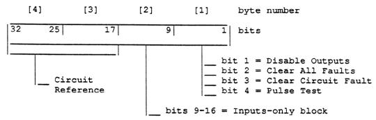
If DIAGNOSTICS ENABLED is set to Y on the CPU Configuration Setup Menu, the CPU also reserves Bus Controller output reference bits 33 through 48 for diagnostics information. Of these additional 16 bits, only bit 33 and bit 34 are used:
