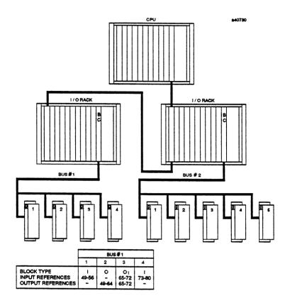
The first Bus Controller is assigned to references 1 through 48. Block 1 on bus 1 is a discrete 8-circuit block with inputs only. It is assigned to Reference Number 0049, reserving 8 input references (10049-10056). Because the block is configured for inputs only, outputs O0049-O0056 are not reserved; they can be used by other blocks.
