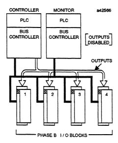
A device that is assigned as a monitor should have all its outputs disabled. This can be done using a Write Configuration command in the program or by setting the Bus Controller DIP switch. If a Bus Controller is used as a monitor, it cannot be located in the same CPU as any other Bus Controllers on the same bus. Otherwise, the CPU would receive input data from both Bus Controllers for the same references, and parity errors could result.
