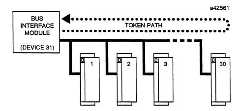
During a bus scan, the Bus Controller automatically:
