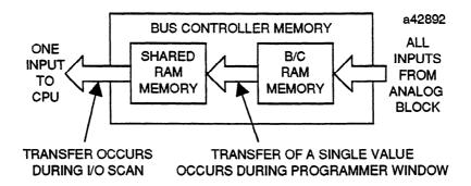
During the I/O scan portion of the CPU sweep, one input per analog block and its circuit number are picked up by the CPU automatically from the block's assigned input references. On successive CPU sweeps, other inputs from the block overwrite the same input references. As explained in chapter 3, logic must be used to copy the input values into other registers to prevent their being constantly overwritten.
