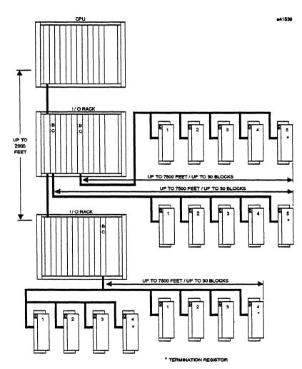
Using More than One Bus Controller on an I/O Chain or Channel
