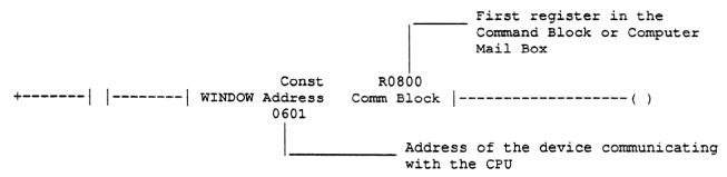
The WINDOW instruction is available with Logicmaster 6 software release 3.0 and later. It requires a CPU with microcode version 110 or greater.
