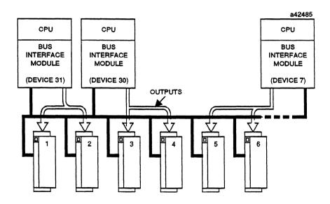
Obtaining Diagnostics from Blocks with Outputs Disabled. Diagnostic messages are automatically sent from a block only to the Bus Controller that is sending or has previously sent it outputs. If the CPU should receive all diagnostics reports from one or more blocks to which outputs are permanently disabled, the Assign Monitor Datagram can be used.
