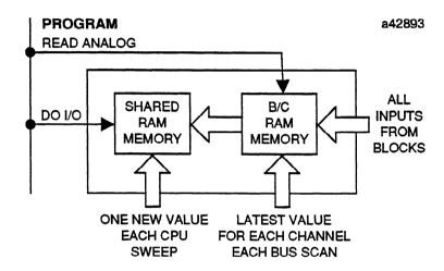
Example program logic for Read Analog Inputs is shown on the next page.
