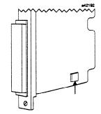
The Bus Controller must be installed downstream of an Auxiliary I/O Module to address the Auxiliary I/O chain or Expanded I/O channels 9 through F.
