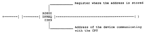
Do not use a DPREQ in a system with Expanded addressing. It would be broadcast to the specified address on all channels. If that address were used for more than one intelligent device (for example, more than one Bus Controller), conflicting replies would be received.
