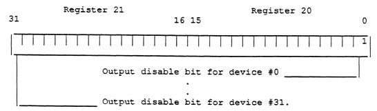
For each bit, a one causes the CPU to read the block's inputs, but not to send outputs. When a bit is 0, outputs are sent to the corresponding Device Number. No more than two CPUs on the same bus should have their outputs enabled to the same blocks. This table can be defaulted to all 0 or all 1 at powerup using the Disable Outputs DIP switch on the Bus Controller (see chapter 2).
