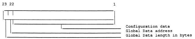
Registers 1-21 contain configuration data, as described earlier (see "Data Returned by a Read Configuration Command to a Bus Controller" in chapter 5). Register 22 must contain the Global Data address.
