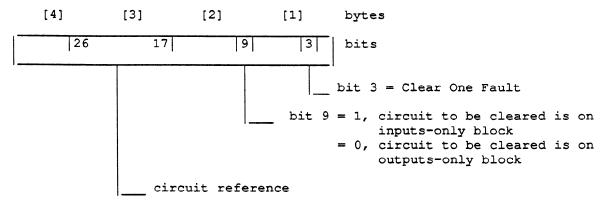
Use bit 9 to indicate whether the block has inputs only or outputs only. Bit 9 will be ignored if the block has both input and output circuits.
