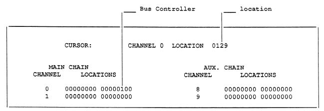
In this example, the CPU would use the 64 I/O references starting at 0129 for diagnostic data for the Bus Controller assigned to Reference Number 0129 in the Main I/O chain. This is explained in chapters 8 and 9. If there were only one Bus Controller in the system, no other entries would be needed.
