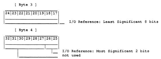
For an analog or RTD block, the circuit is identified by the first six references assigned to the block. The following example shows circuit identification for a 4 Input/2 Output Analog block that starts at I/O references I0801 and O0801):
