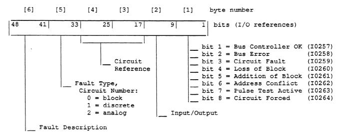
The Bus Controller's 48 assigned input references are I0257 through I0305, so bit 1 is located at I0257.
