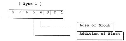
If bit 4 is 1, the Bus Controller has detected the loss of an I/O block that was previously operating. If bit 5 is 1, the Bus Controller has detected the addition of a block to the bus. Either of these bits may be 1 for one CPU sweep for each detected loss or addition; they are never both equal to 1 at the same time. If either of these bits is equal to 1, the other Bus Controller input reference bytes describe the block that was lost or added.
