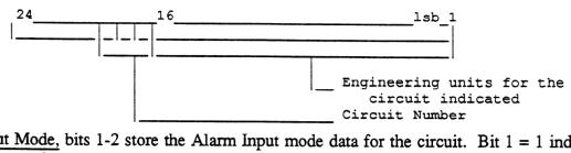
In Alarm Input Mode, bits 1-2 store the Alarm Input mode data for the circuit. Bit 1 = 1 indicates that the current input value exceeds the programmed Low Alarm limit. Bit 2 = 1 indicates that the current input value exceeds the programmed High Alarm limit. If both bits = 0, no alarm limits have been exceeded.
