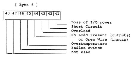
Fault type bits for an analog block:
