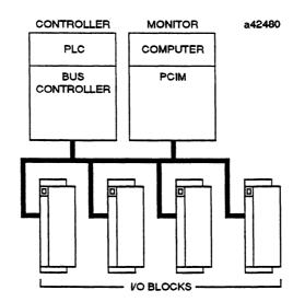
The Assign Monitor Datagram can be sent to phase B Genius I/O blocks only. If sent to phase A blocks or to bus interface modules, the Assign Monitor command has no effect. A complete listing of phase A and phase B Genius devices is located in the Genius I/O System User's Manual (GEK-90486).
