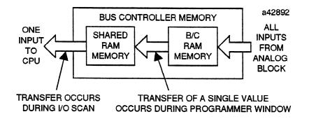
The Bus Controller begins organizing input data from the blocks listed above at the start of the programmer window portion of the CPU sweep, and continues until all the data has been organized. If the program includes DO I/O instructions to obtain the latest data from the block or if the program is very short, program logic should be used to extend the time of the programmer window. This will allow the Bus Controller time to complete the task before the I/O update begins.
