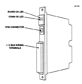
A Bus Controller may be located in the CPU rack or in a regular or High-capacity local I/O rack (that is, a rack communicating with the CPU via a parallel chain). Each Bus Controller draws 20 units of load (one unit = 300mW) at +5 volts. A phase B Bus Controller does not use +12 volts.
