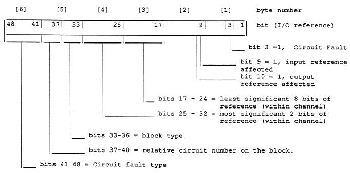
Bits 9 through 16 indicate whether input or output references (or both) are affected. If bit 9 is 1, the circuit is an input. If bit 10 is 1, the circuit is an output. If both are 1, the circuit is an output with feedback, or the fault affects an entire block which is configured as a combination block.
