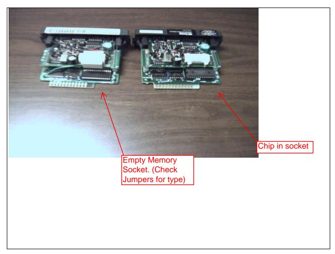
The next point to consider is the pin 1 notch of the chip. If the chip is put in backwards, you fry the board, chip, and possibly the power supply too. In the picture below you see how there is a notch on one side of the chip. Pin one is on the notch side. There is a socket at the base of the CPU card. It should have a picture of how the chip goes on. If it is worn off or missing, the notched side of the chip will be towards the center of the card.
